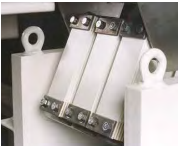
Fiberglass springs attach the base to the trough
